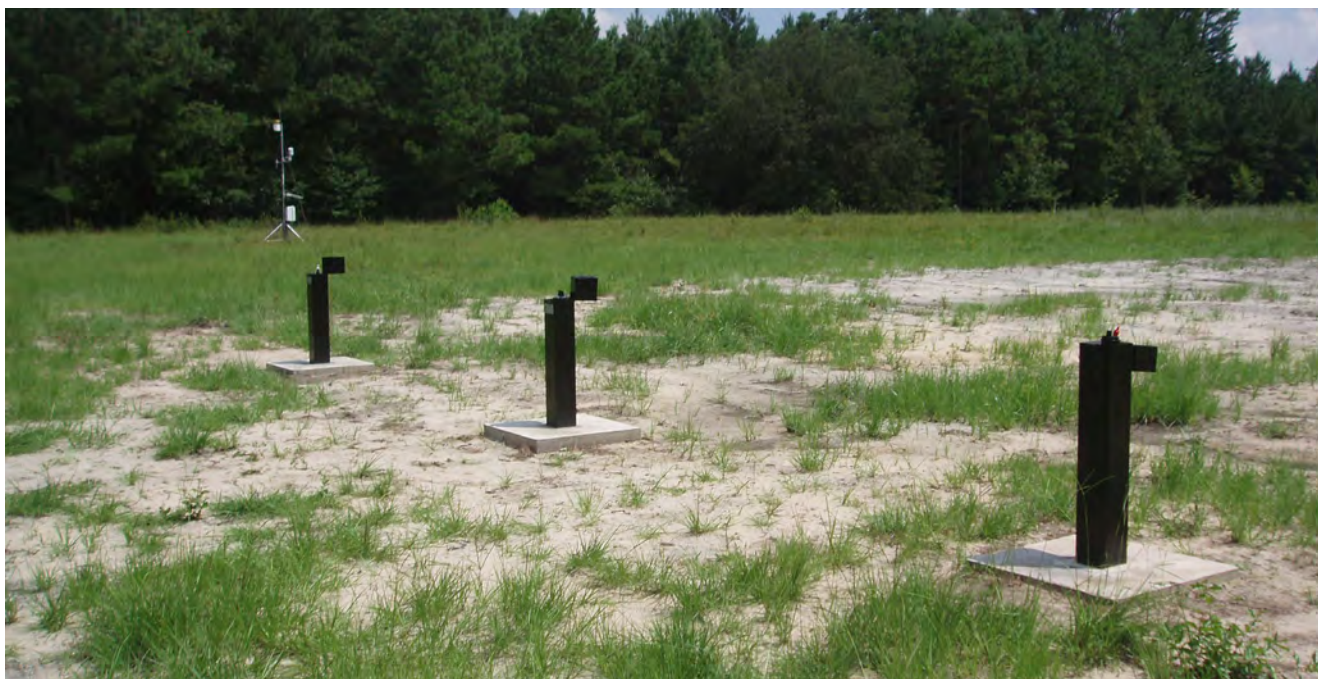
Figure 38. The three completed wells at the Hobcaw site in Georgetown County. In the background is a weather station operated by Clemson University.
