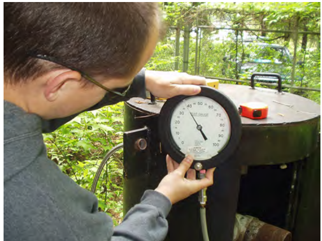
Figure 5. Manual measurement of a water level in a flowing well using a pressure gage.
