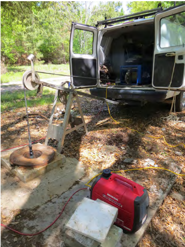
Figure 29. Preparing to run geophysical logs of the Dixie Plantation well. The logging tool is hanging in the well, about to be lowered to the bottom of the well.
