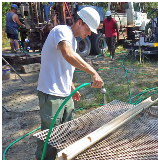
Figure 33. USGS and DNR personnel collecting core samples at the McBee cluster site in June 2014.
