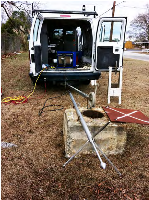
Figure 24. Preparing to run a caliper log of the Williston well (BRN-0078). The logging tool is seen here, out of the well, with its arms fully extended. Inside the well, the arms measure the diameter of the well as the tool is brought up from the bottom of the well.
