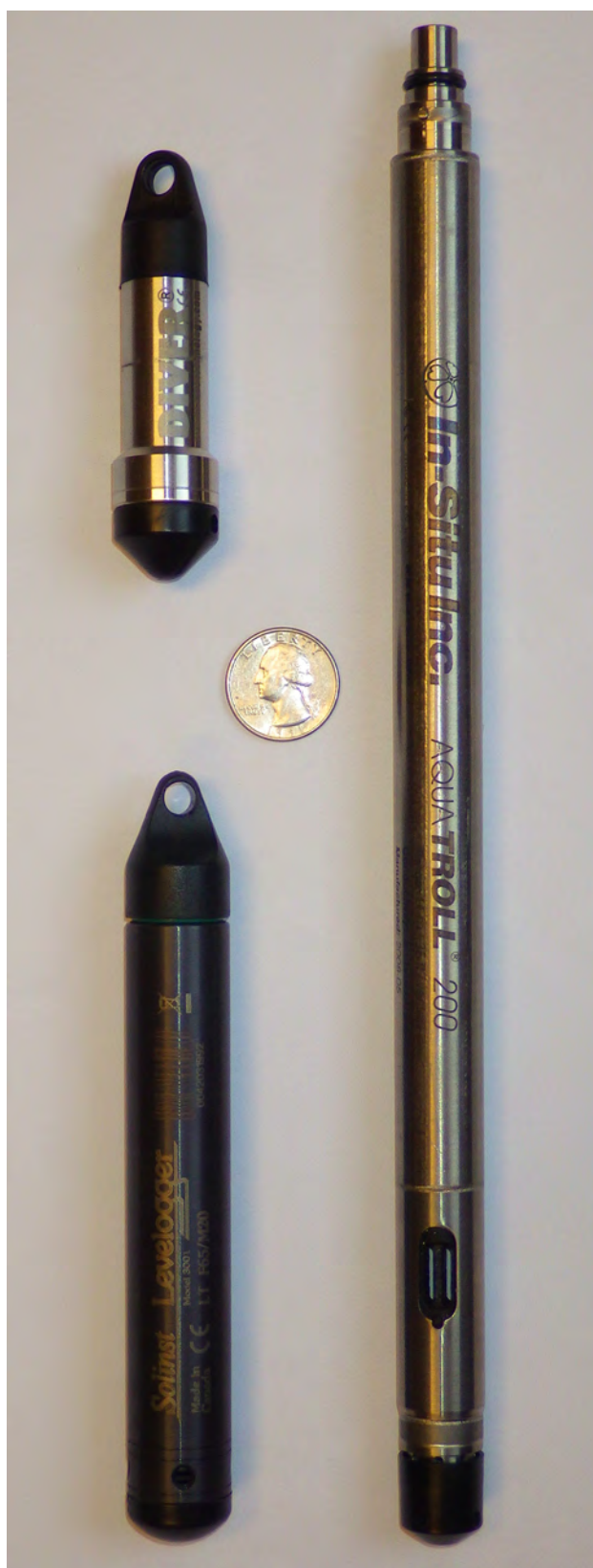
Figure 7. Three ADR water-level probes used in the DNR network: Schlumberger® Diver® (upper left); Solinst® Levelogger® (lower left); and In-Situ® Aqua-Troll® (right), which also measures conductivity.
