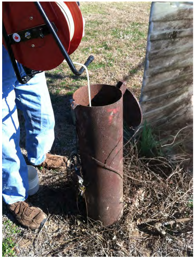
Figure 4. Manual measurement of a water level using an electric tape.
