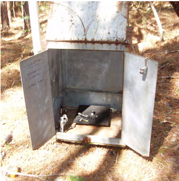
Figure 16. Modern transducers (visible on top of the steel plate, which is covering the well) fit easily inside the metal housing that was constructed to accommodate much bulkier shaft-encoder equipment that was previously used to record water levels in this well (CHN-0101) near Awendaw in Charleston County. DNR took over monitoring of this well in 2012 from the USGS, which had monitored the well since 1980.
