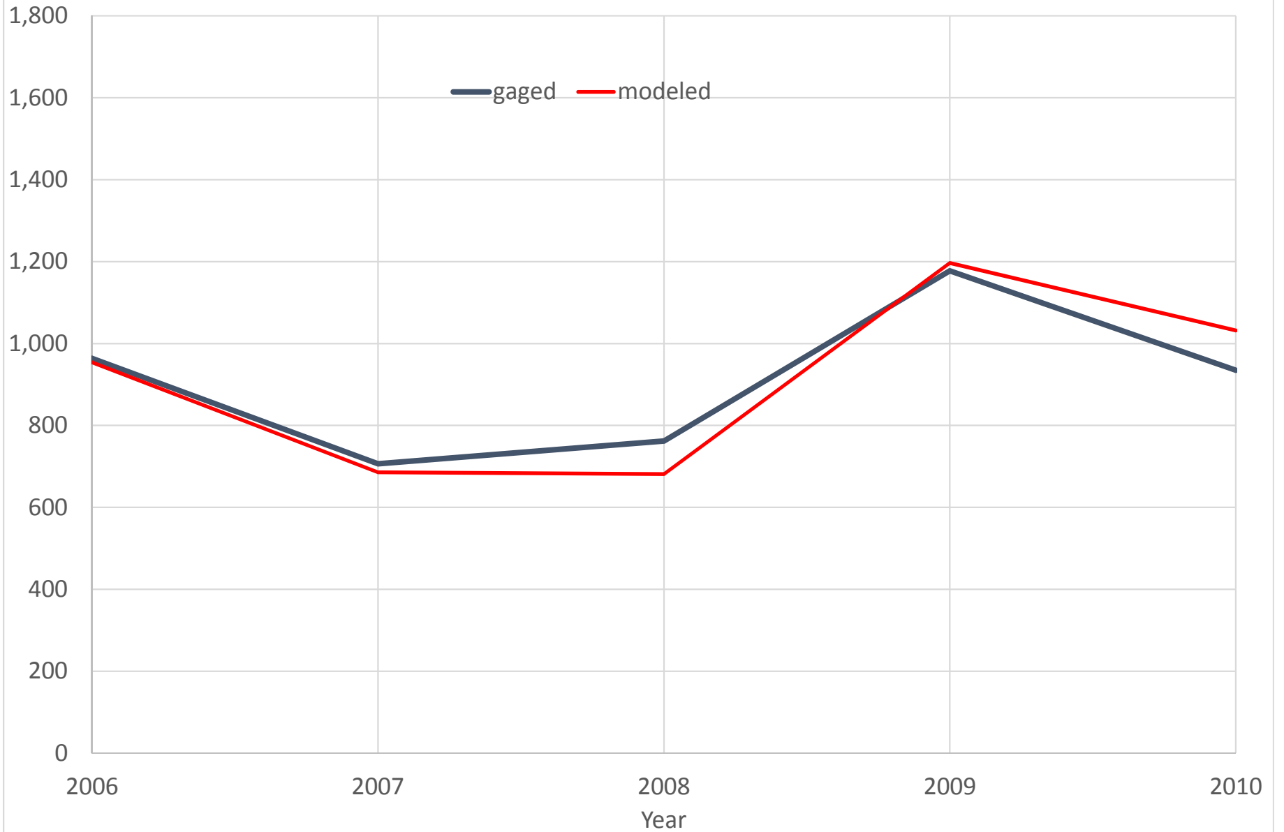
CAT04 (02146000) CATAWBA RIVER NEAR ROCK HILL, SC Annual 7-day Low Flow (CFS)
