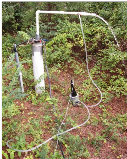
Above: Cluster well being pumped and field tested for field parameters. Right: Water parameter measurement system
