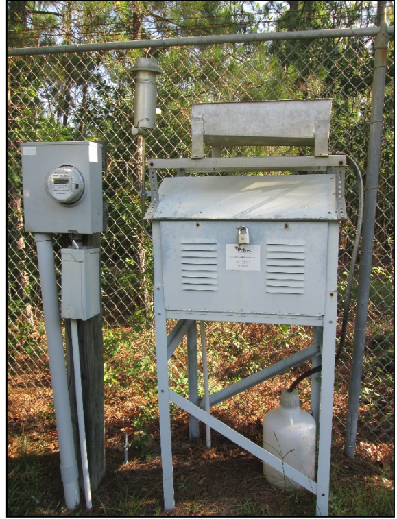
Example of an Air Monitoring Station with Rain Collection Pans and Glass Fiber Filters (on top) and Silica Gel Columns (inside)
