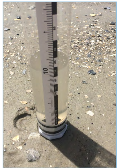
Stationary disk transparency tube as sample water is lowered and disk begins to be visible. Ruler in centimeters for measurement.
