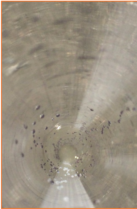
Stationary disk transparency tube as sample water is lowered and disk begins to be visible. Ruler in centimeters for measurement.
