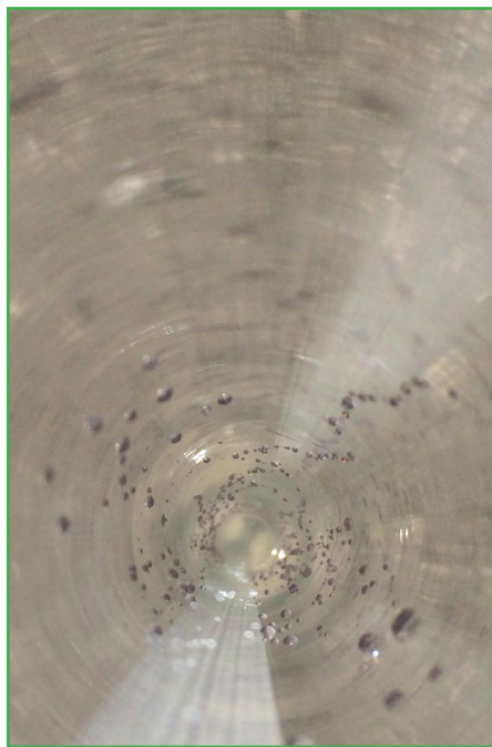
Stationary disk transparency tube as sample water is lowered and disk begins to be visible. Ruler in centimeters for measurement.
