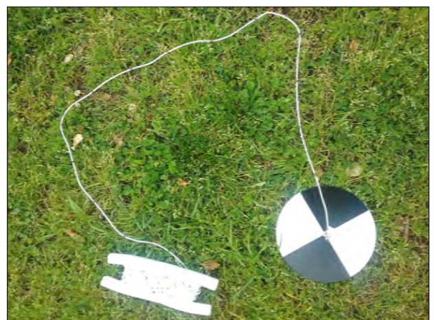
10 cm, 50 cm, and 100 cm markings on SC AAS Kit Secchi disks.
