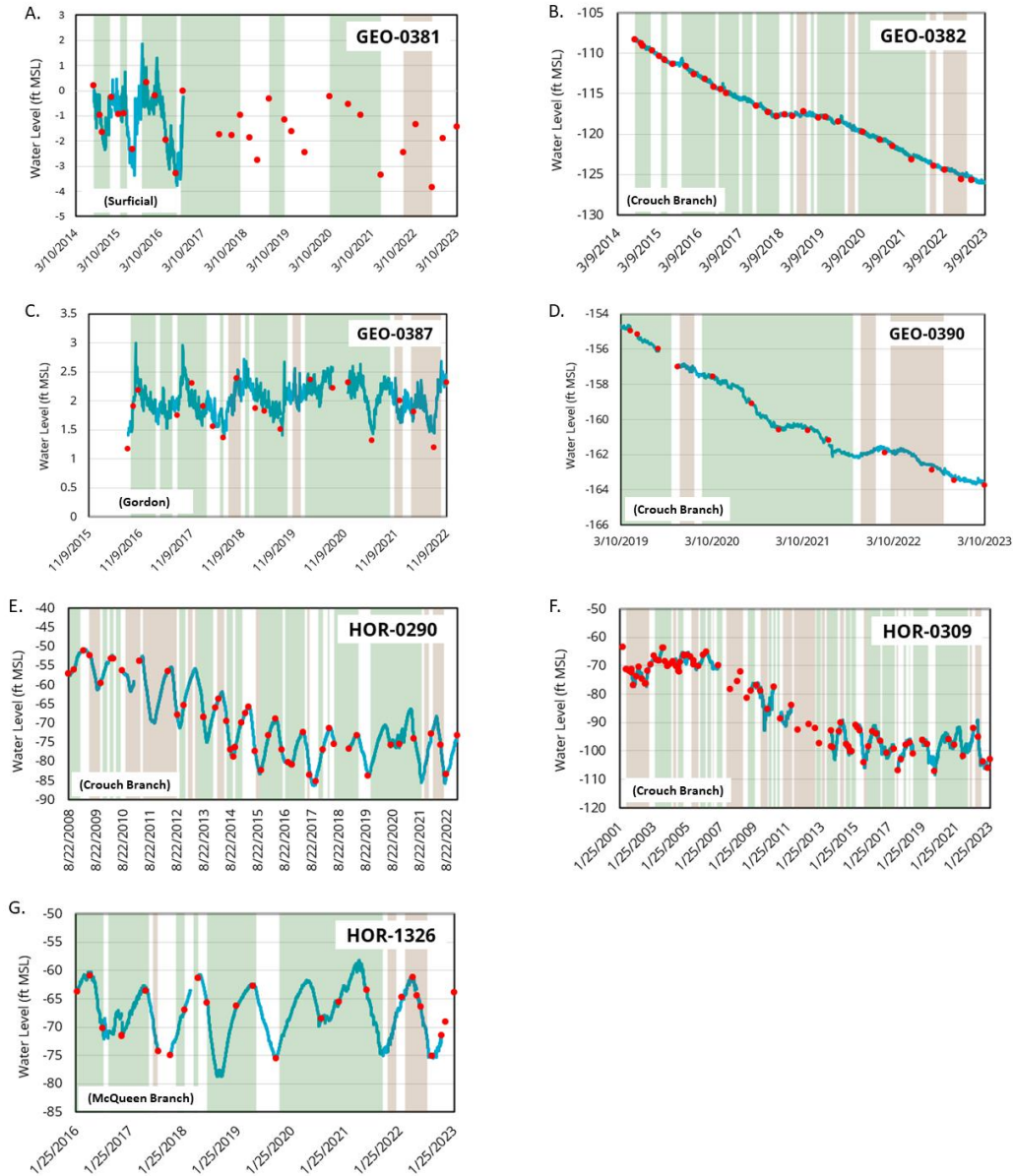
Figure 14. Water level plots from SCDNR monitoring wells in the Waccamaw Area. Water levels are in feet relative to MSL. The blue lines represent automatic data recordings and red dots represent manual water level measurements. The green background indicates wet periods, and the brown background indicates dry periods. http://hydrology.dnr.sc.gov/groundwater-data/ and https://www.drought.gov/states/south-carolina ; accessed March 31, 2023.
